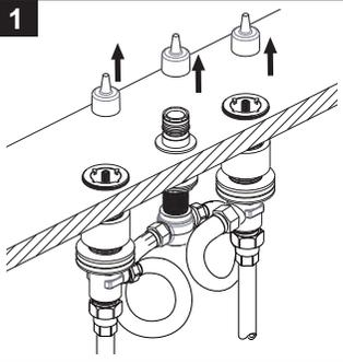
Remove the mud guards from the spout nipple assembly, the hot and cold valves.
