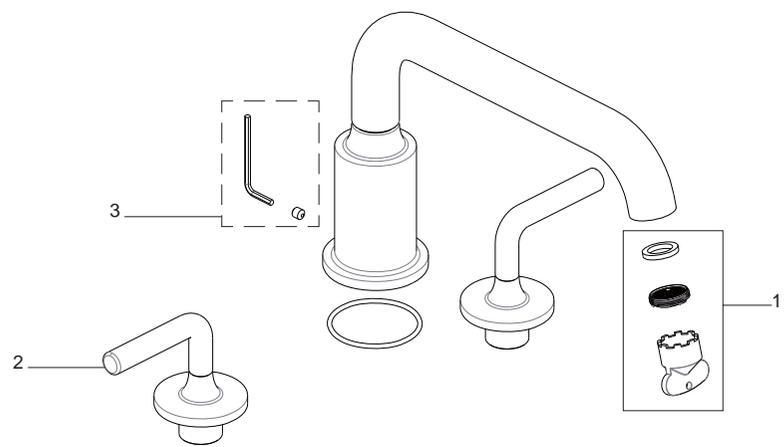
The diagram shows the handle assembly (2) and the aerator (1) with its washer, key, and set screw (3). The aerator is shown in an exploded view, highlighting its internal components.
