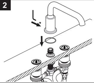
Place the spout "O" ring under the spout and install spout on spout nipple assembly. Be sure the spout is firmly resting on the deck and secure the spout. Secure the spout with the setscrew.
