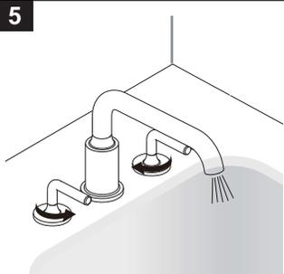
Remove the aerator with key. Turn the faucet handles on full for one minute to flush debris.
